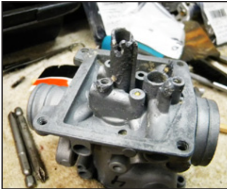
The left one is missing one of the float posts, and the right one...well...time can do terrible things to pot metal...
